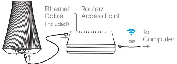
When "LINK" light on speaker turns orange, **unplug the cable**. System will reboot/sync to Wi-Fi® (green light).
