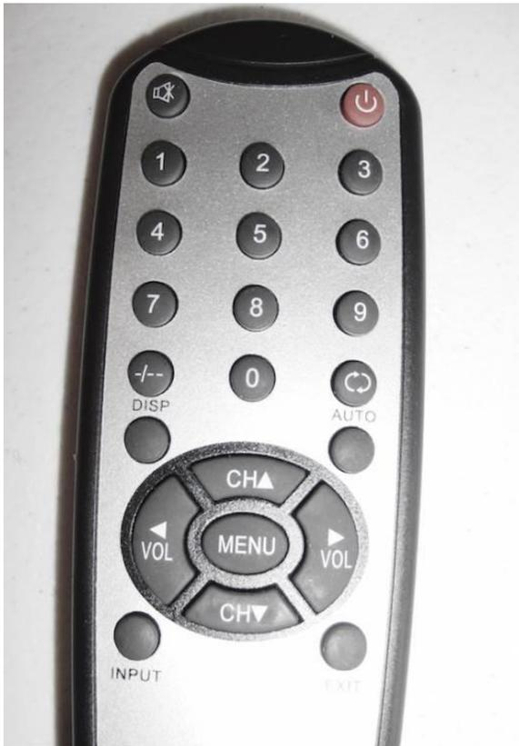
This change can also be made using the remote control (through the USB port or the bottom access hole). Use the **MENU** button, followed by the **VOL** and **CH** buttons to select the Aspect Ratio menu.
