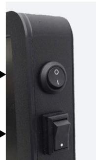
The right-most button on the bottom-front of the unit controls power to the screen. Even if the main power switch is on, this button could prevent you from seeing the screen. The best procedure for using the device is:
