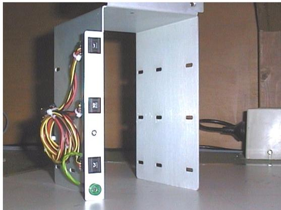
**Drive Bracket Removed From Mainframe**
