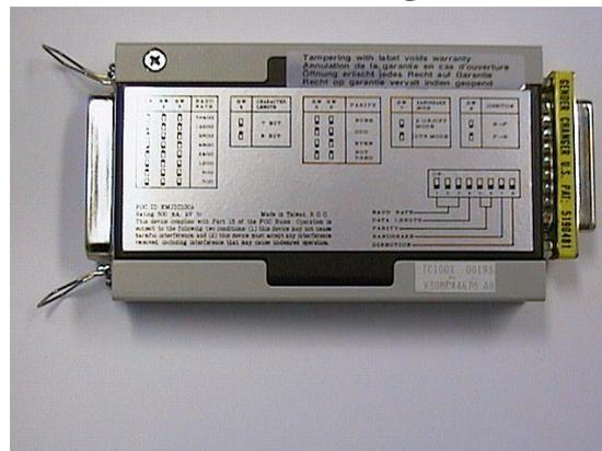
**Primax Side View Showing Correct Switch Settings For MFX**
