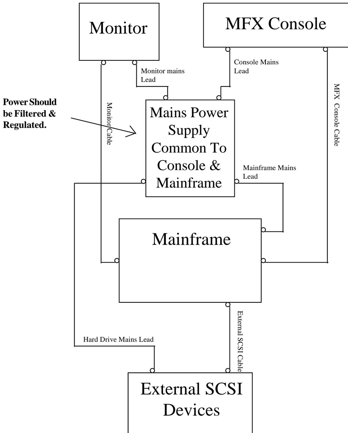
It is strongly advisable that the one source of power be used for both the MFX console and the Mainframe.
