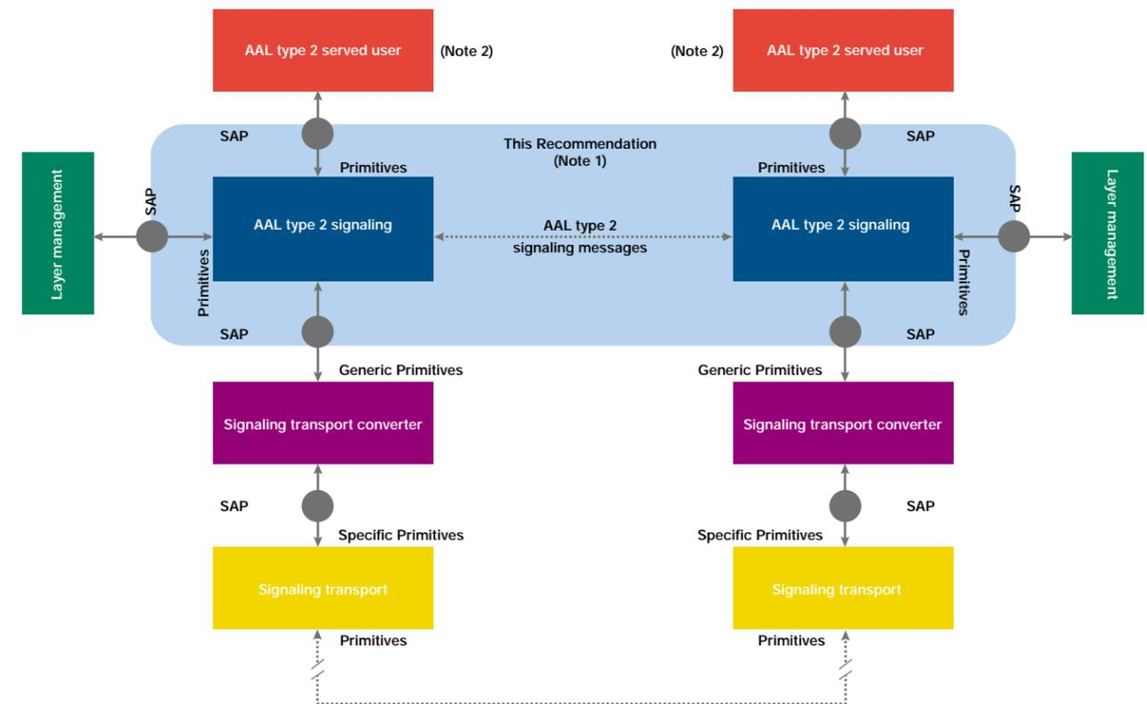
► Figure 10: Protocol structure of AAL2 layer 3
