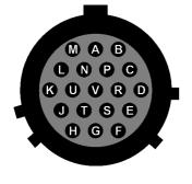
Wiring details for the compatible socket, \*\*\*-14-19S, as seen from the cable end.
