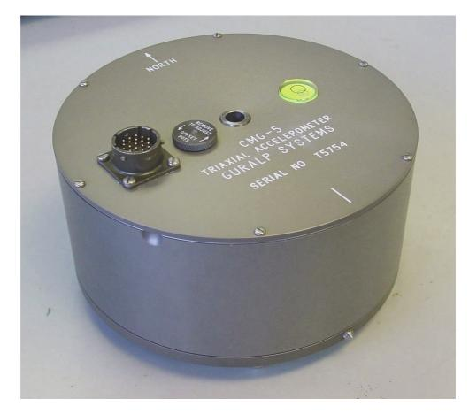
The 5T system combines low-noise components with high feedback loop gain to provide a linear, precision transducer with a very large dynamic range. In order to exploit the whole dynamic range two separate outputs are provided, one with high gain and one with low gain. Nominally, the high gain outputs are set to output a signal 10 times stronger than that from the low gain outputs.
