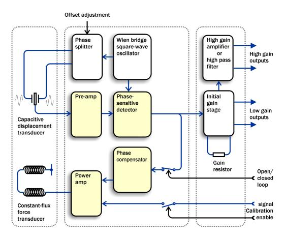
The mass and the capacitor plates are energised by a two-phase transformer driver, forming a differential capacitor. This acts as a capacitive transducer, whose signal is then demodulated with a phasesensitive detector. The accelerometer feedback loop is completed with a feedback loop compensator and a feedback force transducer power amp.
