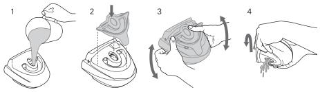
Wash the water chamber, tub plate and tub plate seal in warm water, using a mild detergent. Use the yellow cleaning plug to assist in the cleaning process (see steps 1 to 4). Rinse thoroughly in clean water and allow them to dry away from direct sunlight.
