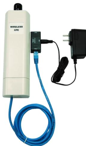
To configure the EX2 Series radio, connect an Ethernet cable to the LAN port on the POE adapter and to a computer. Ensure that the distance between the POE and the radio does not exceed 150ft (45m) when using the supplied 12VDC adapter. Use Tranzeo’s standard 18VDC adapter (purchased separately) when connecting up to 300ft Ethernet cable. If connecting to a hub or switch, a crossover cable may be required.
