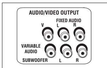
**AUDIO/VIDEO OUTPUTS** Lets you connect an amplifier or audio receiver for improved sound quality or an external video monitor.
