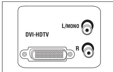
**DVI-HDTV Input** Lets you connect an HD receiver with a DVI output.
