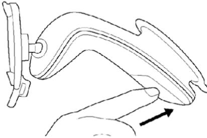
1. Clean the suction cup and that part of the windscreen to which you want to secure the cradle. Both must be dry and free of dirt and grease.
