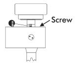
With the aid of a good magnifying glass adjust the needle until it is vertical in the groove (i.e. perpendicular to the record's surface). Ideally this should correspond to the top surface of the cartridge body being parallel to the record surface, but in practice this is often not the case.
