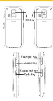
Side top left: Side bottom left: Side top right: Side bottom right: Volume control Radio key Flashlight key Keypad lock key.
