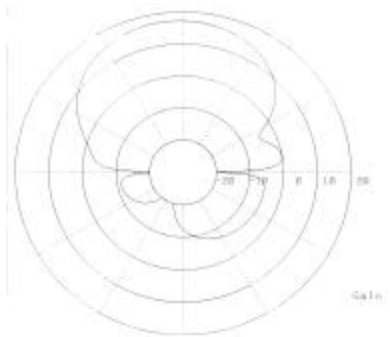
AP Antenna Pattern Azimuth
