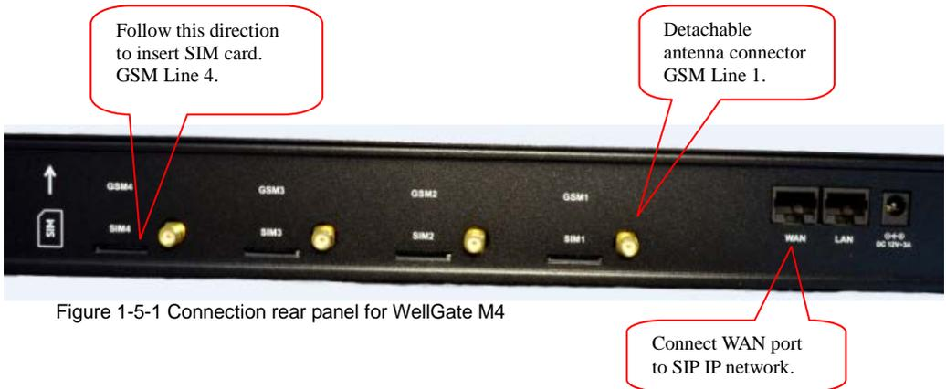
Figure 1-5-1 Connection rear panel for WellGate M4
