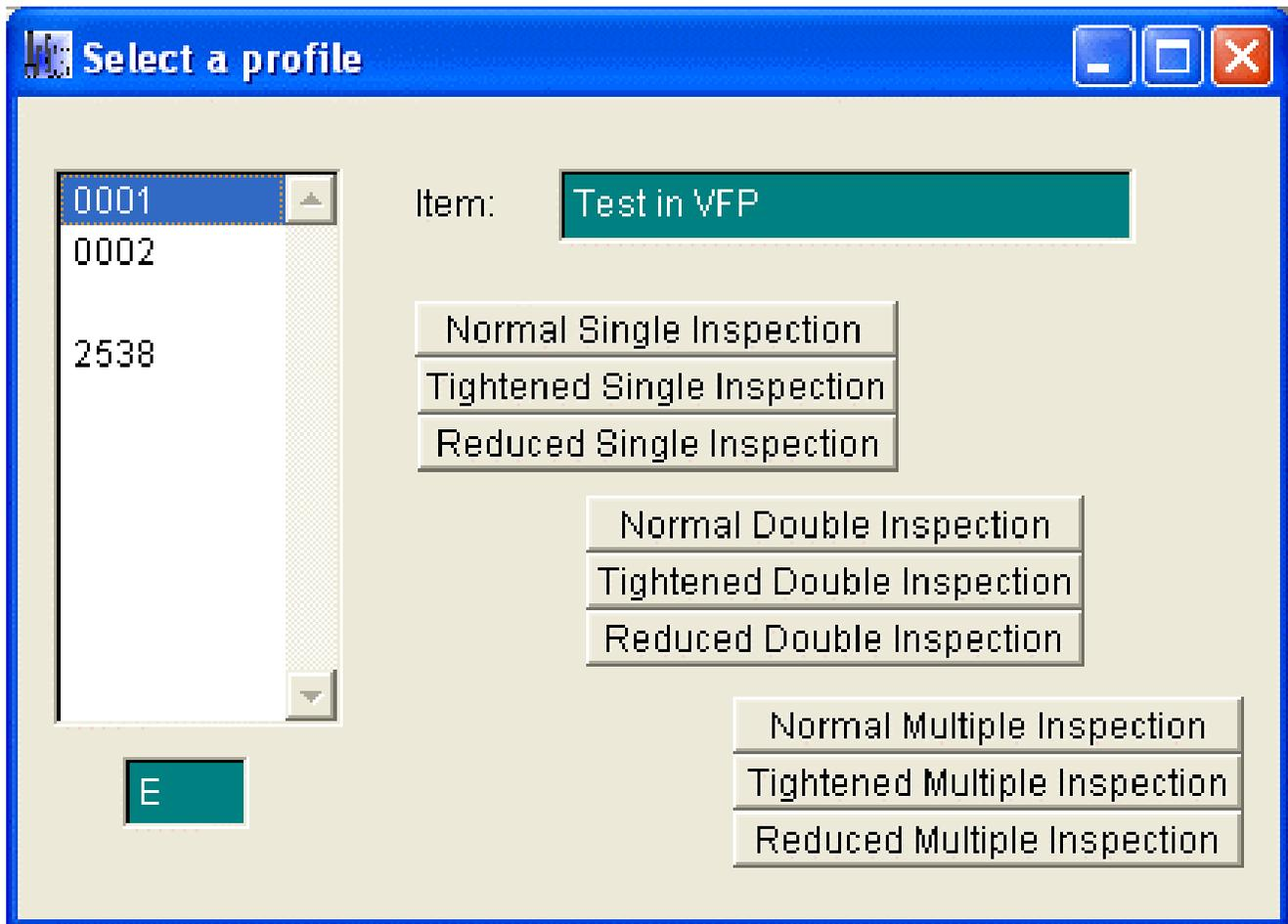
Use the menu slider to select a previously saved sampling profile. Once an item number is selected the **CODE LETTER** is automatically populated in the code letter field located below the menu slider and the item name is automatically displayed.
