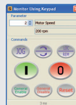
Monitoring and command window using virtual Keypad. Start/Stop function, JOG, local / remote, Reverse and reset
