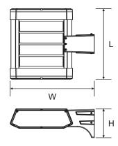
Mounting height≥8m, the maximum projection area of undergoing wind: L(m) x W(m) x 0.5
