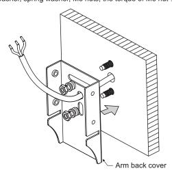
Put 2 pcs M8\*80mm expansion screws into the drilled hole.
