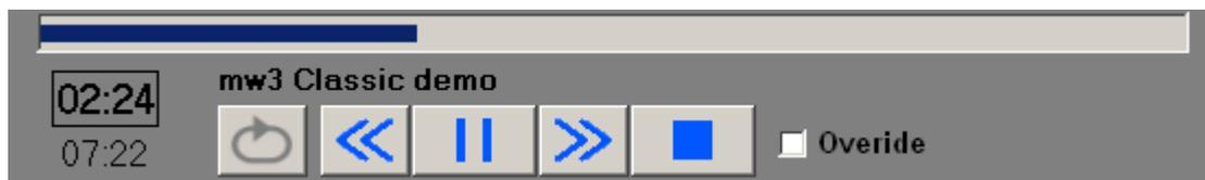
Once playback has started the Pause, Skip Forward, Skip Backwards and Repeat buttons are enabled. Left mouse clicking anywhere on the Progress Bar will skip playback to that time.
