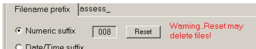
Suppose there was one recording in the sequence you wanted to keep. Simply load it and right click on the number text above the OPEN button. You can then save it as another name, and then use the Reset button to delete all files in the sequence.
