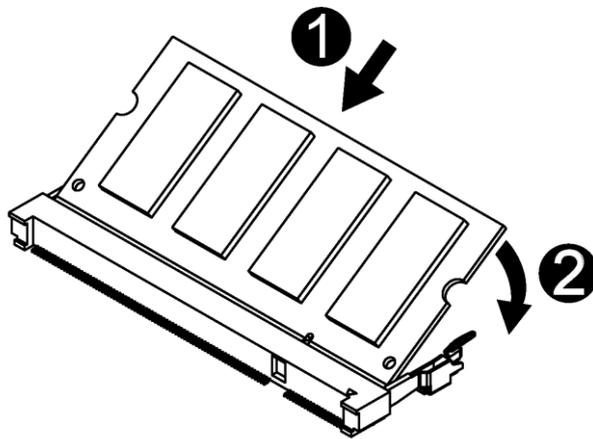
3. To remove the Memory modules, please push the clips outwards, and the memory modules will be automatically disengaged.
