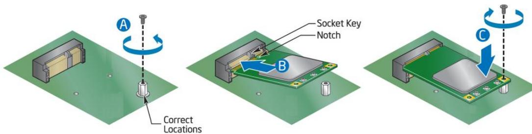
Note: BNX-I61 comes also with one half-sized Mini Card slot, supporting all general half-sized miniPCIe module. Please follow the same procedure for proper installation.
