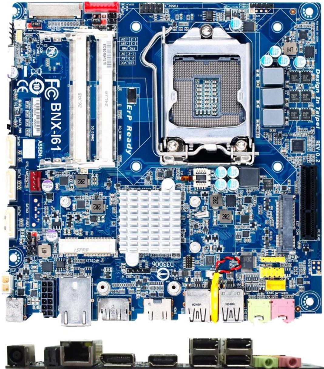
Figure 1.1: Board Layout of BNX-I61
