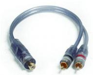
Russell's Tip: Use an RCA (Y) lead to connect both the Left and Right Channel inputs together this gives a 6db level boost to the input of the subwoofer amplifier. The cable can be up to 5M long
