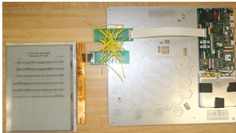
Figure 35: Dual PCB Testing Setup
