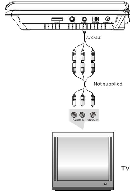
Please use AV cable to connect the machine and the TV. Make sure it is connected correctly.
