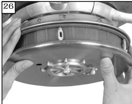
Loosen 3 screws with slots and remove 2 without slot. Place switch housing over 3 screws and twist into place. Tighten the 3 screws with slots and replace and tighten the 2 removed.
