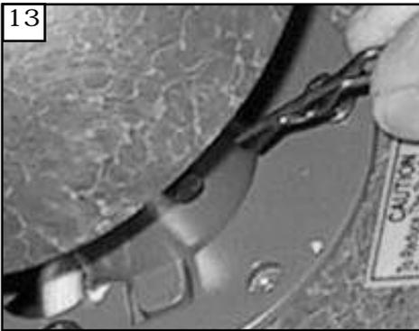
13 Install keeper pin into cross pin.
