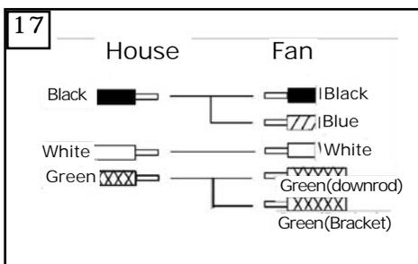
17 For pul chain controls, follow diagram above. Make sure that all exposed wiring is secured inside wire nuts. Note: Wires from house may vary in color and may not include ground wire. After wiring is complete, gently push wires into junction box with wire nuts pointing upward. Refer to point 3 of safety tips.
