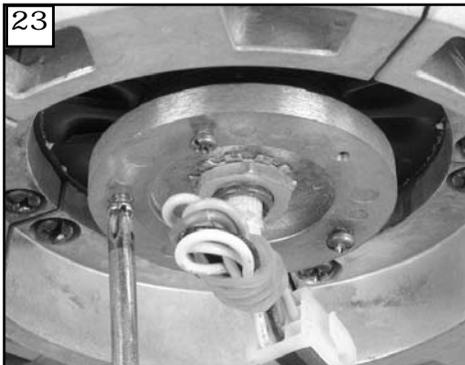
Loosen 4 screws with slots and remove the other screw.
