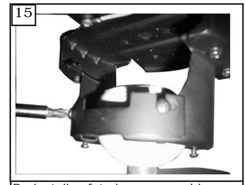
15 Re-install safety bar removed in step. 3 by placing safety bar on screws, sliding into place, and tightening the 2 screws.
