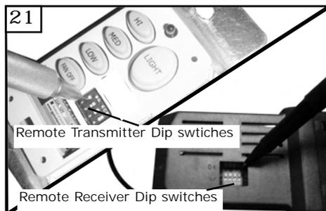
21 Set dip switches on the Remote Transmitter and Remote Receiver to the same settings. This must be done so the units will communicate properly. If you have other fans you can set to control from one transmitter by setting both receivers the same as the transmitter. If you have more than one fan with remote. You can set the dip switches to different positions to have separate control.
