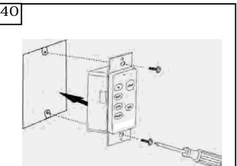
Install wall control unit to outlet box using machine screws provided.
