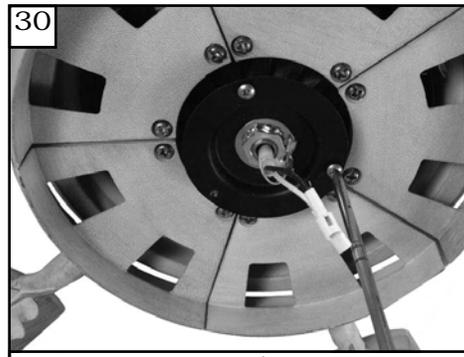
30 Loosen 2 screws and remove 1 screw. Save screw removed.
