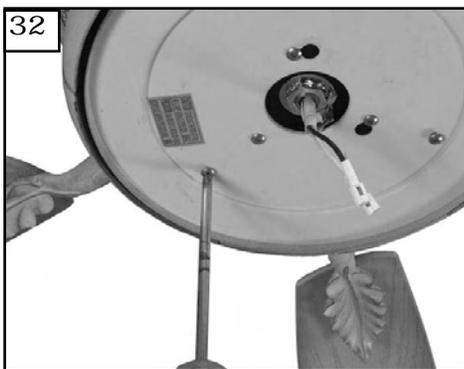
Loosen 3 screw on light plate as shown.
