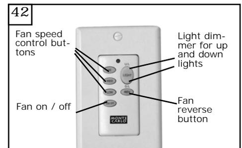
To control fan speed select from High, Medium or low speed buttons. To turn the fan off press the Fan on / off button. To dim upper lights press and hold U/L button. To dim Lower lights press and hold D/L button. To turn off either up or down light press and quickly release either U/L or D/L button. Press button marked REV to reverse the rotation direction of the fan blades
