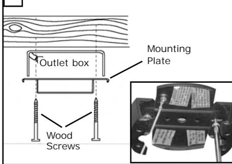
Secure mounting plate directly to a joist from the building structure via the two knock out holes on the outlet box. Use only the appropriate wood screws and washers included with your fan. Caution: Wood screws must go through into the building joist.
