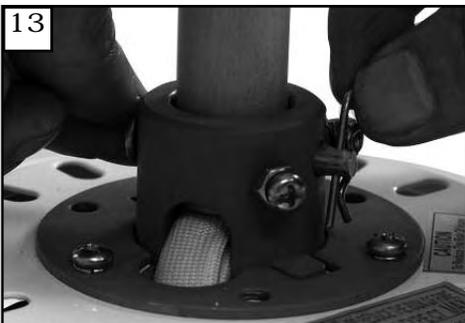
Thread wiring through downrod. Align hole in downrod with hole in yoke and install cross pin. Install downrod into yoke. Install keeper into cross pin.
