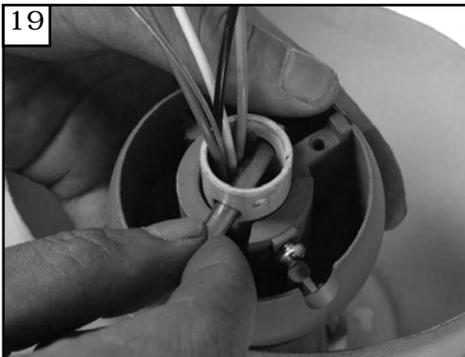
19 Place ball on downrod. Replace pin removed earlier and pull ball up so that the pin fits in the notches in the ball.
