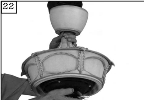
22 Raise fan with downrod assembled to the ceiling bracket and hang fan assembly. Be sure to rotate the downrod ball so that the notch in the bracket engages the slot in the ball.
