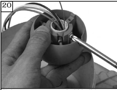
20 Tighten set screw to hold ball in place.
