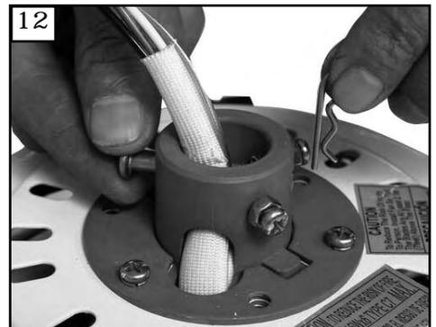
Remove keeper from cross pin and then cross pin from yoke. Replace keeper on cross pin and save.
