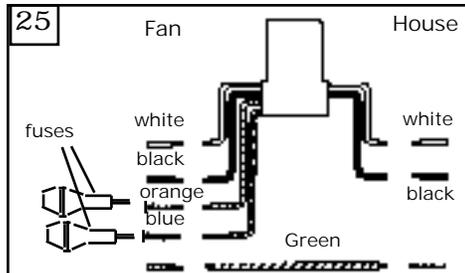
25 Make wiring connections as indicated above. White from fan to white from remote marked N. Orange from fan to Orange from remote marked Light/up. Blue from fan to blue from remote marked down light. Black from fan to Black from remote marked L. White from house to white from remote marked AC N. Black from house to Black from remote marked AC L. Connect all green ground wires to Ground wire from House.
