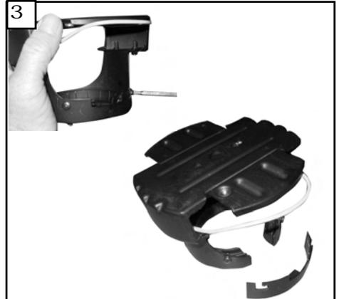
Remove Safety bar from mounting bracket by loosening screws, sliding bar to side, and lifting it off the 2 screws.
