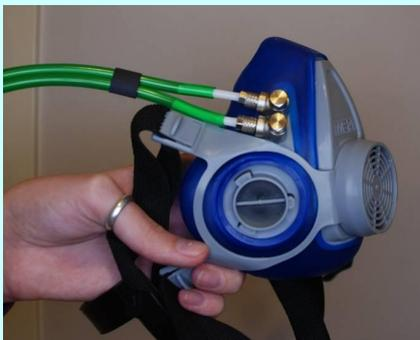
An Oxelerate mask with dosage tube connections and dosage tube connected.
