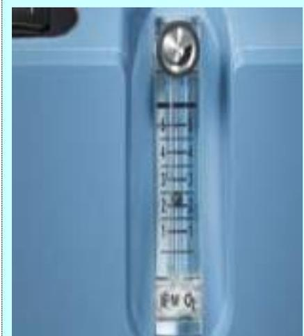
Oxygen concentration level is properly set. The Oxygen flow control on the EverFlo should be at or below 2 LPM.
