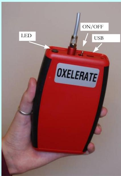
**Switch on** the Oxelerate Athlete Unit. The pin of the power switch shall point towards the breathing sensing port. In the picture the switch is in the “OFF” position
