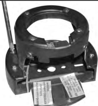
Remove the 4 screws attaching the Mounting neck to the mounting plate. Retain the 4 screws for re-assembly.
