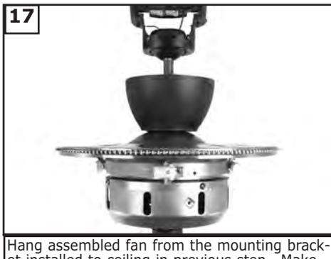
17 Hang assembled fan from the mounting bracket installed to ceiling in previous step. Make sure the fan is hanging straight. Rotate fan until the tab on the Mounting bracket engages the slot on the Downrod Ball. This must be done to prevent the fan body from rotating when the blades are in motion.
