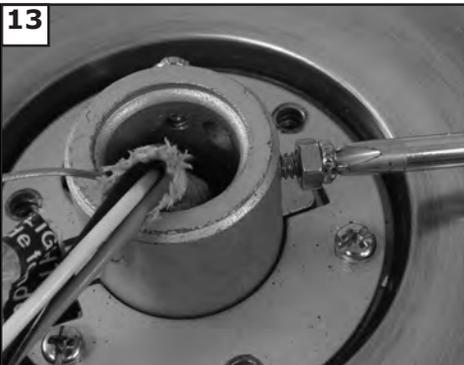
13 Loosen 2 set screws with lock nuts in yoke till you can not feel them on inside of yoke.
