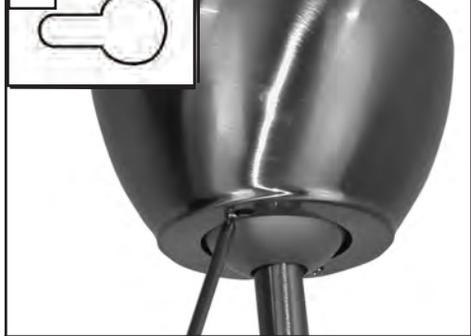
Lift Canopy to ceiling aligning the key hole slots with the screws on the bottom of the Mounting bracket. Rotate the canopy Counter Clockwise to lock in place. Tighten the screws to secure the Canopy. See inset for Keyhole shape
