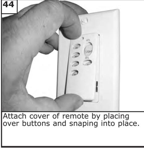
Attach cover of remote by placing over buttons and snapping into place.
