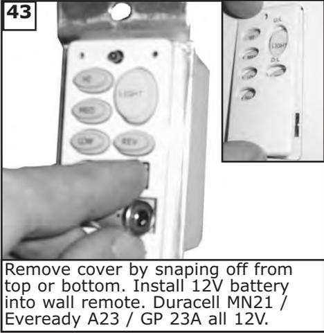
Remove cover by snapping off from top or bottom. Install 12V battery into wall remote. Duracell MN21 / Eveready A23 / GP 23A all 12V.
