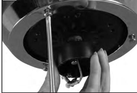
Loosen 2 screws with key hole slots and remove 1 screw.
