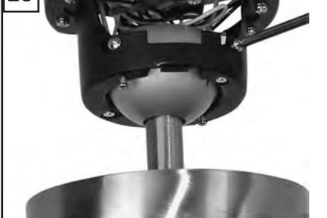
Re-install safety bar removed in step 3 by placing safety bar on screws, sliding into place, and tightening the 2 screws.
