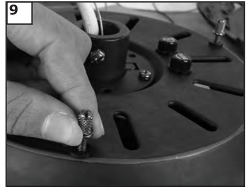
9 Loosen 3 thumb screws with key hole slots.
