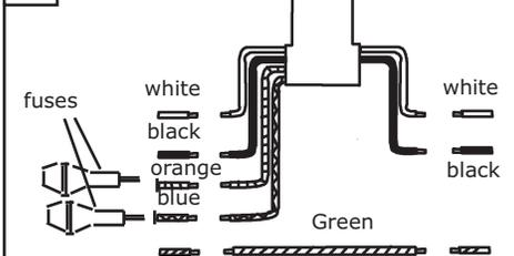
Make wiring connections as indicated above. White from fan to white from remote marked N. Orange from fan to Orange from remote marked Light/up. Blue from fan to blue from remote marked down light. Black from fan to Black from remote marked L. White from house to white from remote marked AC N. Black from house to Black from remote marked AC L. Connect all green ground wires to Ground wire from House.
