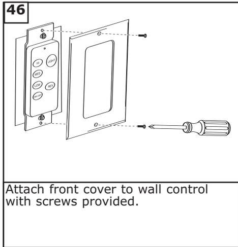
Attach front cover to wall control with screws provided.
