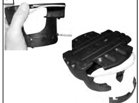
Remove Safety bar from mounting bracket by loosening screws, sliding bar to side, and lifting it off the 2 screws.
