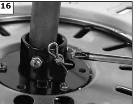
16 Tighten set screws and lock nuts to secure downrod in place.
