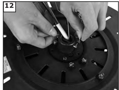
12 Remove keeper from pin and then pin from yoke and save.
