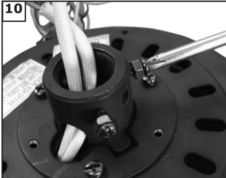
10 Loosen 2 set screws with lock nuts in yoke till you can not feel them on inside of yoke.
