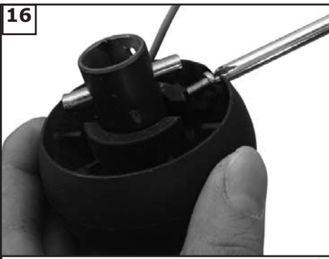
16 Loosen screw, remove cross pin, and remove downrod ball. Save for re-installation.
