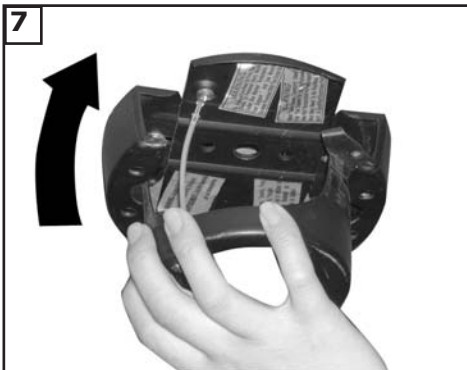
7 Lift mounting neck to mounting Plate and align screws.
