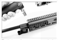
The bottom rail screws are secured using a thread locker. Using a heat source such as a Chef's Torch, heat the screws until the thread lock releases.
