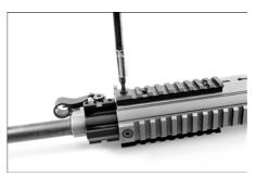
Tighten the (4) rear barrel extension screws and (2) forward barrel extension screws in an alternating sequence until snug.
