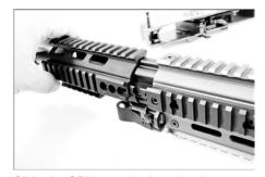
Slide the SRX onto the barrel yoke as shown. The QD Sling swivel points will be toward the rear of the weapon.
