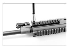
Loosen the (2) Forward Barrel Screws by turning counter clockwise until the screws reach the end of their travel.
