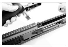
Best results will be acheived if a directed flame can be used to focus the heat onto the screw instead of all over the rail.
