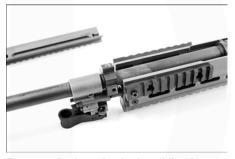
Remove the barrel yoke by sliding it foward toward the gas block.
