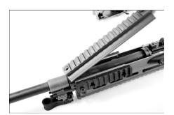
**AFTER THE RAIL HAS COOLED** remove the bottom rail by lifting up and away.
