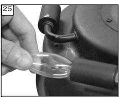
Install 6 x 15 watt candelabra torpedo shape bulbs.
