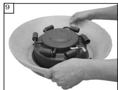
Lower upper glass disk onto fan housing and align 3 holes in glass with 3 holes in fan housing.
