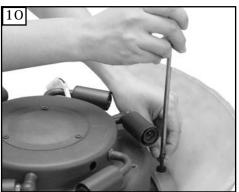
Install 3 screws to hold glass to fan housing. Do not overtighten as this could crack the glass.
