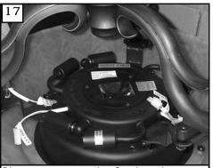
Place arms over the fan housing. Make sure the arms with electrical connection plugs are next to the plugs on the fan housing.
