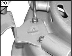
Align holes in arch arm and slot for tab with holes and tab on fan body. Start all screws in the arch arm brackets.
