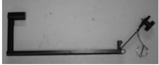
(2) Remove locking pin on the pivoting arm
