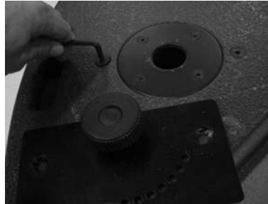
(2) Remove ETRI adapter plate attachment screws (5 mm allen key)
