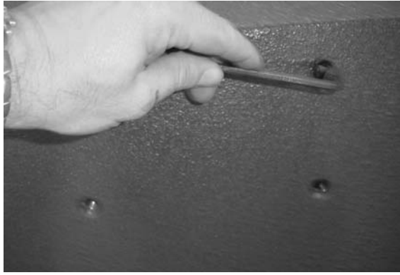
(1) Remove Omnimount attachment screws (5 mm allen key)
