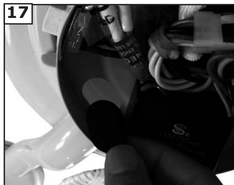
17 After installation of all blades you must replace the rubber grommet to ensure no water leakage through to switch housing.
