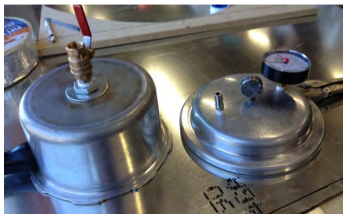
Figure 23 – Pressure Vessel after Modifications
