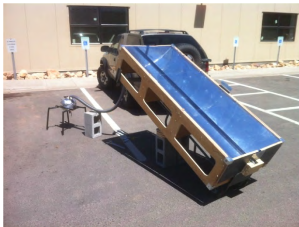
Figure 17 – Completed Solar Autoclave
