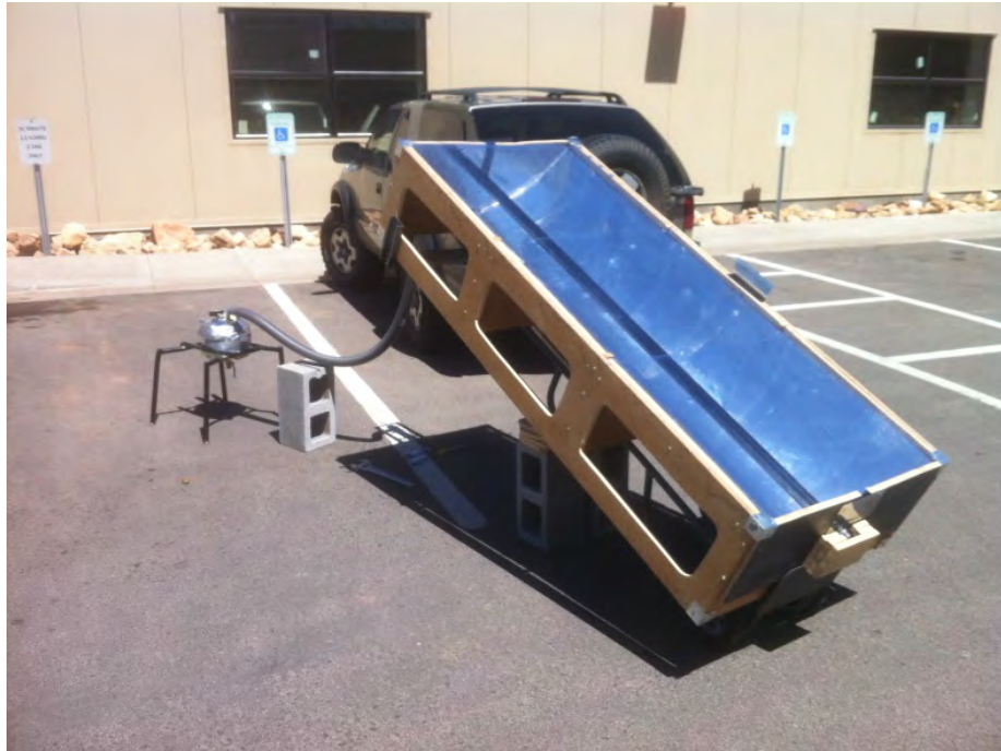
Figure 1 – Solar Autoclave for Rural Areas
