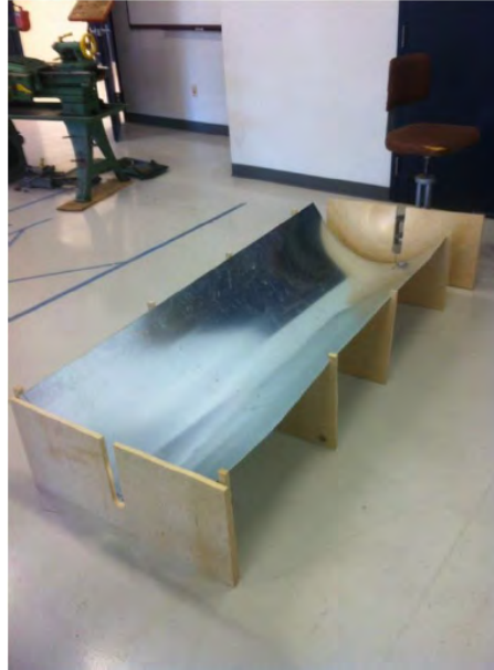
Figure 16 – Parabolic Trough during Construction
