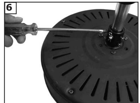
**6** Tighten the 2 Set screws on the Yoke once the downrod is in place. Check motor for shipping stabilizers and remove if present.
