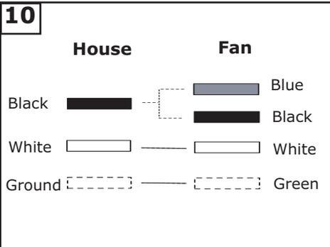
10 Connect black and blue wire from fan to Black or (Hot) wire from house. Connect White wire from Fan to White (Neutral) wire from house. Connect Ground leads from mounting bracket and downrod to Ground lead from house. **Refer to Safety Tips section of manual.**
