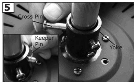
**5** Loosen the 2 set screws in yoke for downrod to slip into yoke. Insert downrod into yoke on top of the Fan Body. Align the hole in the Downrod with the hole in the Yoke. Insert the Pin through the Yoke and Downrod until the point appears on the other side. Install the Keeper Pin
