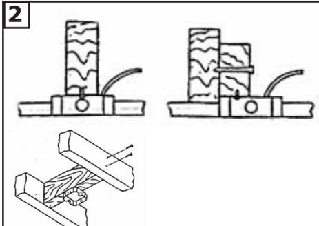
**2** Before installing this fan make sure the outlet box is properly installed to the house structure. To reduce the risk of fire, electric shock, or personal injury, mount to outlet box or supporting system acceptable for fan support. (Mounting must support at least 35 lbs.)
