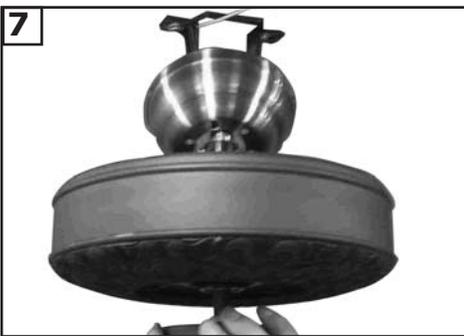
7 Hang assembled fan from the mounting bracket installed to ceiling in previous step. Make sure the fan is hanging straight. Rotate fan until the tab on the Mounting bracket engages the slot on the Downrod Ball. This must be done to prevent the fan body from rotating when the blades are in motion.
