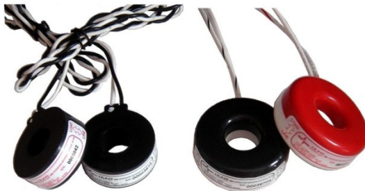
Figure 9: IMS solid core CTs
