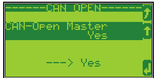
Figure 5-8: Display screen - configure CAN interface
