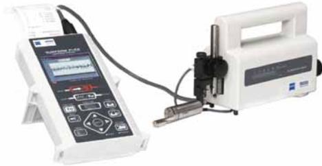
Model combination with small genuine type 50mm tracing driver of S130A. Small tracing driver, available skidless measurement and waviness measurement. Achieve class highest straightness accuracy  $3\mu\text{m}/50\text{mm}$  Easy levelling adjustment by tilting support function.
