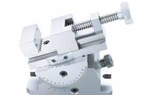
Bench vise can rotate and swivel in 2 axis with a jaw width of 70 mm and a span width of 80 mm. The tilting area is +/- 45°. The rotary area is 360°. The rotatable bench vise is made of steel and delivered with the required fastening material. The bench vise can be mounted directly to the Surfcom.
