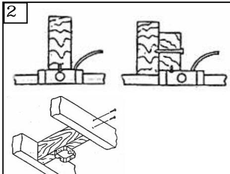
2 Before installing this fan make sure the outlet box is properly installed to the house structure. To reduce the risk of fire, electric shock, or personal injury, mount to outlet box or supporting system acceptable for fan support. (Mounting must support at least 35 lbs.(16 kg.)).
