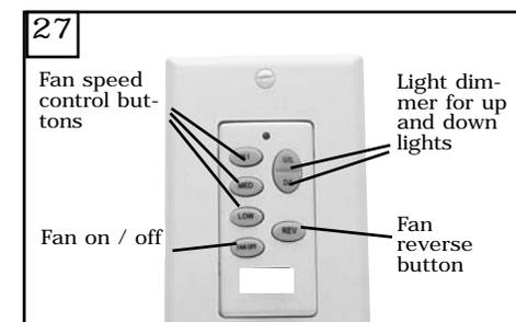
To control fan speed select from High, Medium or low speed buttons. To turn the fan off press the Fan on / off button. To dim upper lights press and hold U/L button. To dim Lower lights press and hold D/L button. To turn off either up or down light press and quickly release either U/L or D/L button. Press button marked REV to reverse the rotation direction of the fan blades
