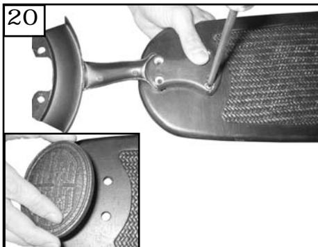
Place medallion on decorative side of blade and blade bracket to other side of blade and attach using the blade bracket screws and washers provided.
