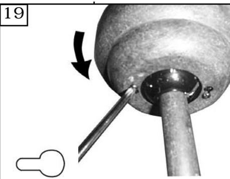
Lift Canopy to ceiling aligning the key hole slots with the screws on the bottom of the Mounting bracket. Rotate the canopy Counter Clockwise to lock in place. Tighten the screws to secure the Canopy. See inset for Keyhole shape
