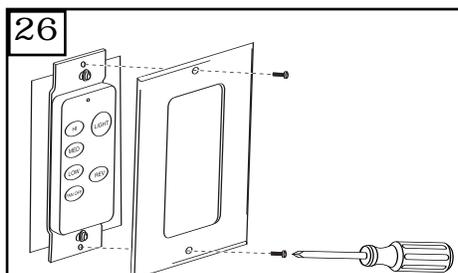
Attach front cover to wall control with screws provided.
