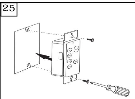
Install wall control unit to outlet box using machine screws provided.
