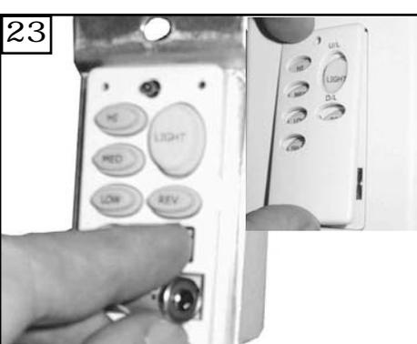
Remove cover by snapping off from top or bottom. Install 12V battery into wall remote. Duracell MN21 / Eveready A23 / GP 23A all 12V.
