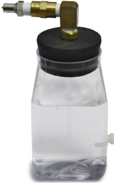
Figure 2.7 - Stopper/Lixit Valve Assembly
