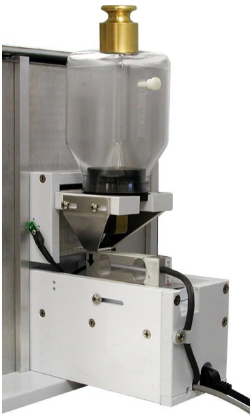
Figure 3.6 - Bottle with Calibration Weight
