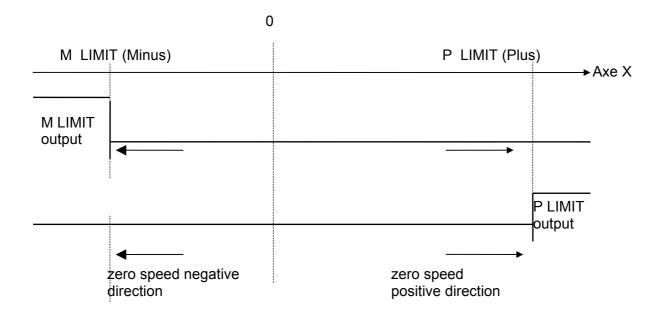
**ATTENTION:** The software limits are cross-referenced to the position origin and therefor related to the origin setting.
