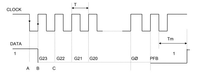
The external clock is at level 1 between two position measurements.
