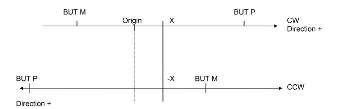
The mechanical position of the PLUS and MINUS LIMITS is therefore reversed.
