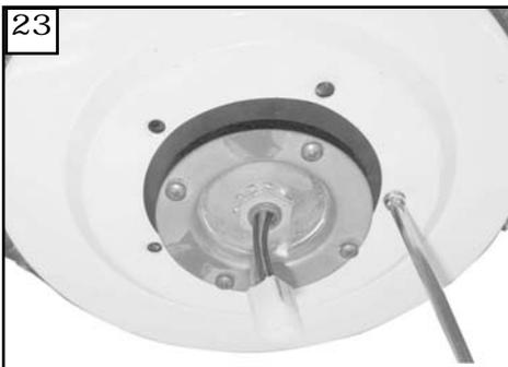
23 Remove the steel motor stabilizing plate and discard.
