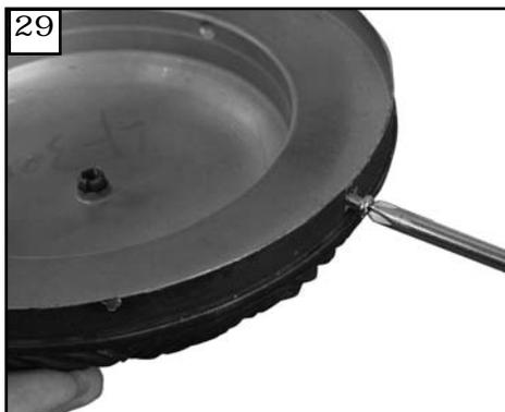
29 Remove 4 screws and save to install switch housing.
