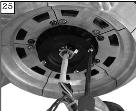
25 Loosen 3 screws with key slots and remove 1 screw without slot from motor plate and save screw.
