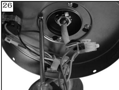
26 Install switch housing plate by twisting plate with key hole slots into place. Replace screw removed and tighten the 4 screws securely.
