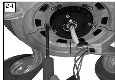
24 The screws, washers, and motor pads are pre-installed to the blade holders. Attach blade assembly to motor and tighten screws securely.
