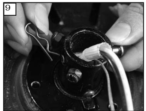
9 Remove keeper from pin. Remove pin replace keeper and save.
