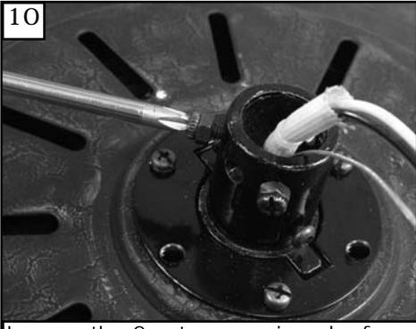
10 Loosen the 2 set screws in yoke for downrod to slip into yoke.
