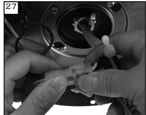
27 Connect plug from fan to switch house plug.
