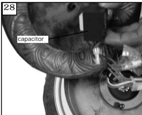
28 Remove the double sided tape from capacitor and stick capacitor to switch housing.
