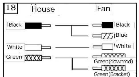
18 For pullchain controls, follow diagram above. Make sure that all exposed wiring is secured inside wire nuts. Note: Wires from house may vary in color and may not include ground wire. After wiring is complete, gently push wires into junction box with wire nuts pointing upward. Refer to point 3 of safety tips.
