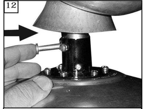
12 Insert downrod into motor yoke. Next, insert clevis pin through yoke and downrod.
