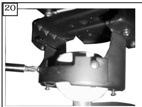
20 Re-install safety bar removed in step. 3 by placing safety bar on screws, sliding into place, and tightening the 2 screws.
