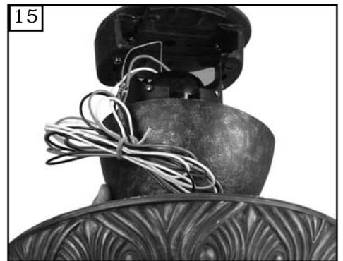
15 Carefully lift fan assembly onto mounting bracket. Rotate fan so that the notch on the ball engages the ridge in the mounting bracket. This will allow hands-free wiring.
