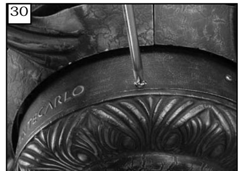
30 Install the switch housing using the 4 screws previously removed.
