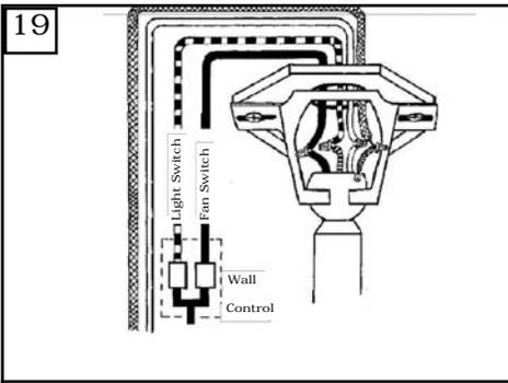
19 For control of fan and optional light from wall location, follow diagram above. NOTE: A professional electrician is recommended for this type of installation.
