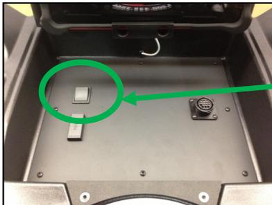
Turn the system power ON. The power switch is located in the iPad recess, near the fuse location.
