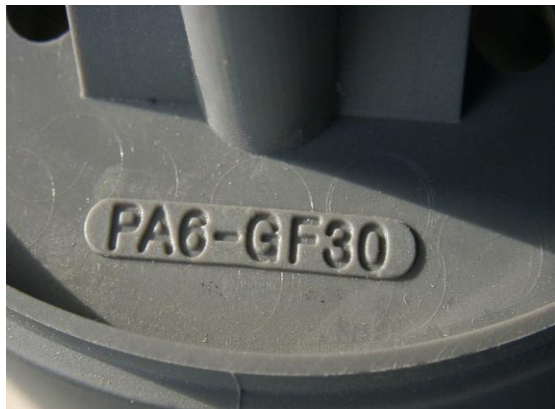
Figure 4. Nylon 6 + 30% Glass fiber
