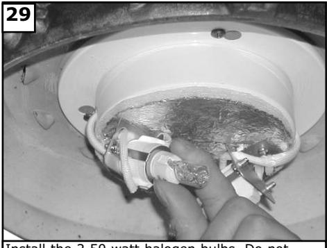
Install the 2 50 watt halogen bulbs. Do not touch bulb surface as oily residue from skin can cause the bulb to explode.
