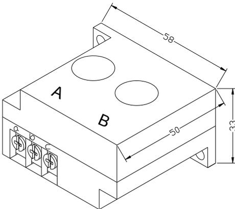
Structure dimensions of CT (φ10 through hole)
