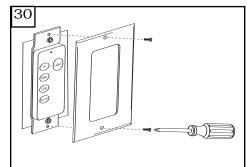
Attach front cover to wall control with screws provided.
