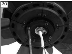
Loosen 3 screws with key slots and remove the 1 screw with closed slot. Save screw removed.
