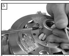
Loosen lock nuts and screws on yoke till you can not feel screw on inside of yoke.
