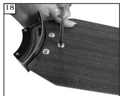
Attach blade arms to blades using the blade arm screws and washers provided.
