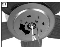
Twist lower cover plate into place by twisting in direction of arrow.
