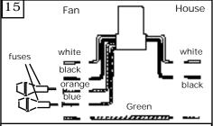
Make wiring connections as indicated above. White from fan to white from remote marked N. Orange from fan to Orange from remote marked Light/up. Blue from fan to blue from remote marked down light. Black from fan to Black from remote marked L. White from house to white from remote marked AC N. Black from house to Black from remote marked AC L. Connect all green ground wires to Ground wire from House.
