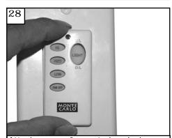
Attach cover of remote by placing over buttons and snaping into place.
