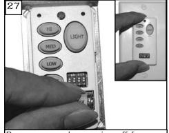
Remove cover by snaping off from top or bottom. Install 12V battery into wall remote. Duracell MN21 / Eveready A23 / GP 23A all 12V.
