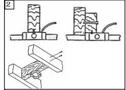
Before installing this fan make sure the outlet box is properly installed to the house structure. To reduce the risk of fire, electric shock, or personal injury, mount to outlet box or supporting system acceptable for fan support. (Mounting must support at least 35 lbs.(16 kg.)).
