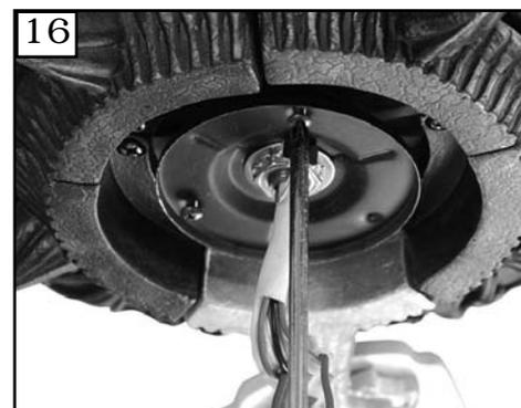
16 Loosen 2 screws and remove 1 screw from motor plate and save screw.
