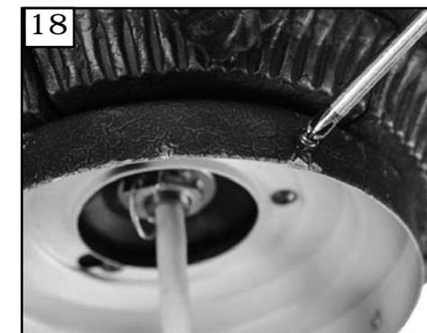
18 Remove 4 screws around light plate. Save screws.
