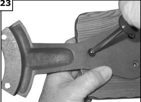
Place blade arms onto the other side of the blade and aligning holes. Insert screws with fabric washers through the holes and tighten securely.
