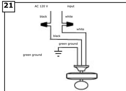
Make wiring connections as shown black wire from house to black wire from fan. White wire from house to white wire from fan. Connect all green ground wires to ground wire from house. Refer to diagram above.
