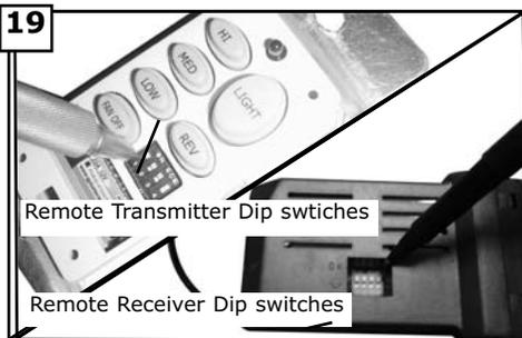
Set dip switches on the Remote Transmitter and Remote Receiver to the same settings. This must be done so the units will communicate properly. If you have other fans you can set to control from one transmitter by setting both receivers the same as the transmitter. If you have more than one fan with remote. You can set the dip switches to different positions to have separate control.
