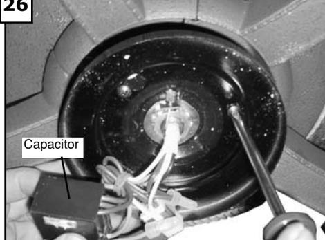
Tighten the three screws securely holding the plate for the switch housing. Remove the double sided tape from capacitor and stick capacitor to plate.
