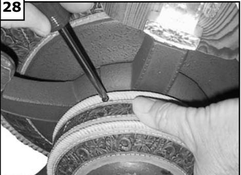
After attaching blades; install the switch housing with the three screws previously removed.
