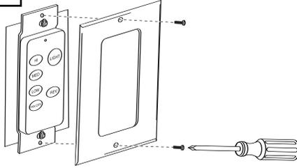
Attach front cover to wall control with screws provided.
