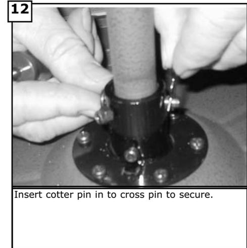
Insert cotter pin in to cross pin to secure.
