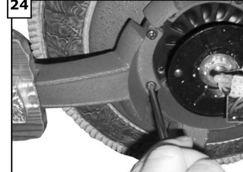
Check the motor for plastic shipping stabilizer tabs, and remove them if they are present. Attach blade assembly to motor by tighten screws securely.
