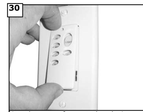
Attach cover of remote by placing over buttons and snapping into place.
