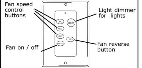
To control fan speed select from High, Medium or low speed buttons. To turn the fan off press the Fan on / off button. To dim lights press and hold button. To turn off light press and quickly release button. Press button marked REV to reverse the rotation direction of the fan blades
