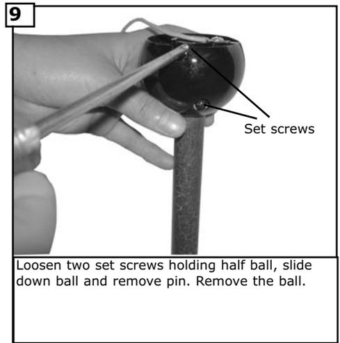
Loosen two set screws holding half ball, slide down ball and remove pin. Remove the ball.
