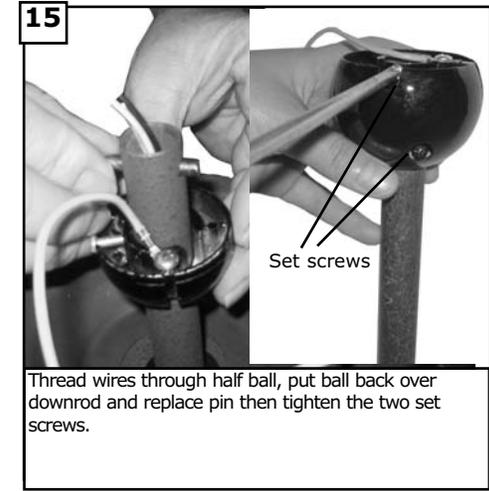
Thread wires through half ball, put ball back over downrod and replace pin then tighten the two set screws.
