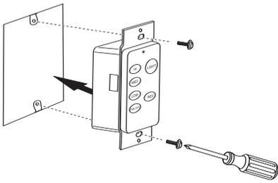
Install wall control unit to outlet box using machine screws provided.
