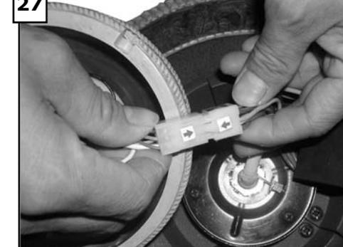
Make sure to connect the plug from remote to the plug coming from fan body according to the arrows indicated on the plugs, otherwise the remote will be damaged.
