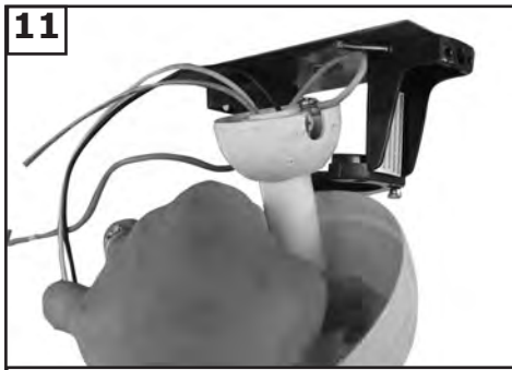
11 Hang assembled fan from the mounting bracket installed to ceiling in previous step. Make sure the fan is hanging straight. Rotate fan until the tab on the Mounting bracket engages the slot on the Downrod Ball. This must be done to prevent the fan body from rotating when the blades are in motion.
