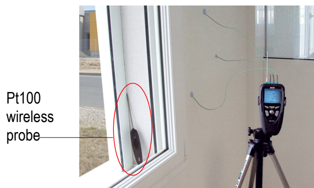
(3) Positioning wireless probe
