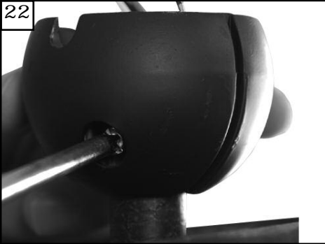
22 Tighten set screw to hold ball in place.
