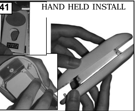
41 HAND HELD INSTALL Place face plate over battery compartment and buttons. Place remote over 2 pins on front cover. Attach cover of remote by placing over 4 pins and snapping into place.
