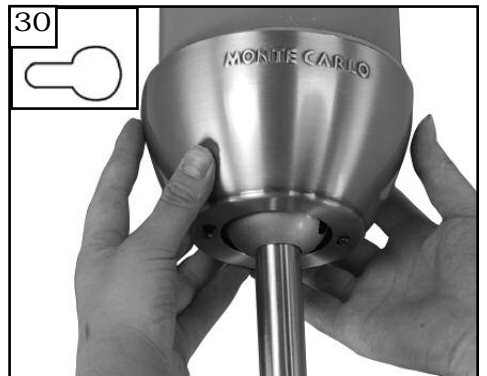
30 Lift canopy to ceiling aligning the key hole with the screws on the bottom of the mounting bracket. Rotate the canopy counter clockwise to lock in place. Tighten the screws to secure the canopy. See inset for keyhole shape
