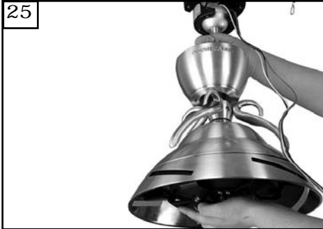
25 Raise fan with downrod assembled to the ceiling bracket and hang fan assembly. Be sure to rotate the downrod ball so that the notch in the bracket engages the slot in the ball.
