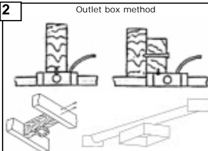
**Warning**—Risk of fire, electric shock, or personal injury. The fan in this box may be either directly supported from a structural framing member of a building and/or may be mounted to an outlet box marked acceptable for fan support of 31.8 kg(70lbs) or less. Most outlet boxes commonly used for the support of luminaires may not be acceptable for fan support and may need to be replaced. Consult a qualified electrician if in doubt.
