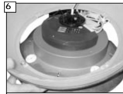
Lower upper glass disc onto fan housing and align 4 holes in glass with 4 holes in fan housing.
