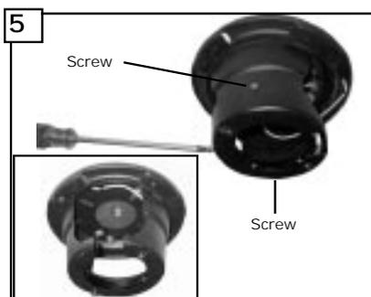
Take out screw in back that holds mount ring and save. Check the two screws on each side and tighten. Mount ring turns clockwise to open.
