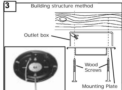
Secure mounting plate directly to a joist from the building structure via the two knock out holes on the outlet box. Use only the appropriate wood screws and washers included with your fan. Caution: Wood screws must go through into the building joist.
